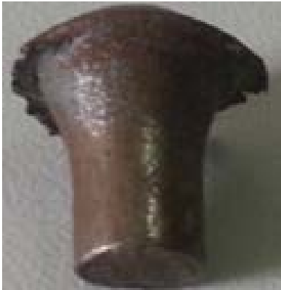
Comparison of bullet core between simulation and experiment at the speed of 720m/s
