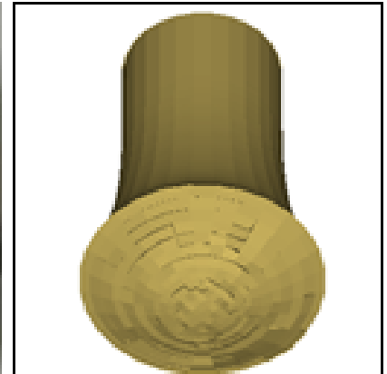
Comparison of bullet core between simulation and experiment at the speed of 720m/s
