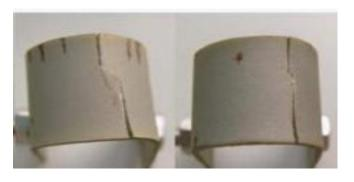
☐ The possibility of hydrogen-induced delayed fracture (HDF) of hot stamping parts exits, which will decrease the car's passive safety. More and more carmakers care about it!
