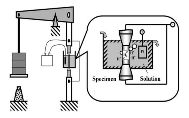
Diagrammatic sketch for constant load test
