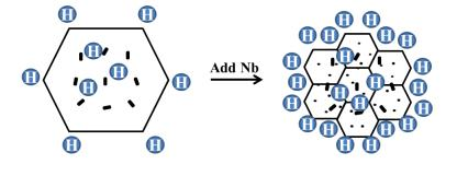
☐ Some trapping, such as second phases particles( TiC and Fe<sub>3</sub>C), interact strongly with hydrogen and lead to the uniformly distributed of hydrogen in steel. NbC may also belongs to this trapping.
