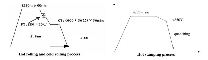
$\square$  Then the specimens were heated up into austenite region at 930 °C, held for 3 min, and deformed while water quenching.
