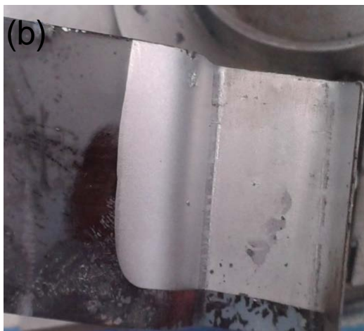
Al-Si coating stamping piece (a) Cold stamping (b) Hot stamping at 850°C
